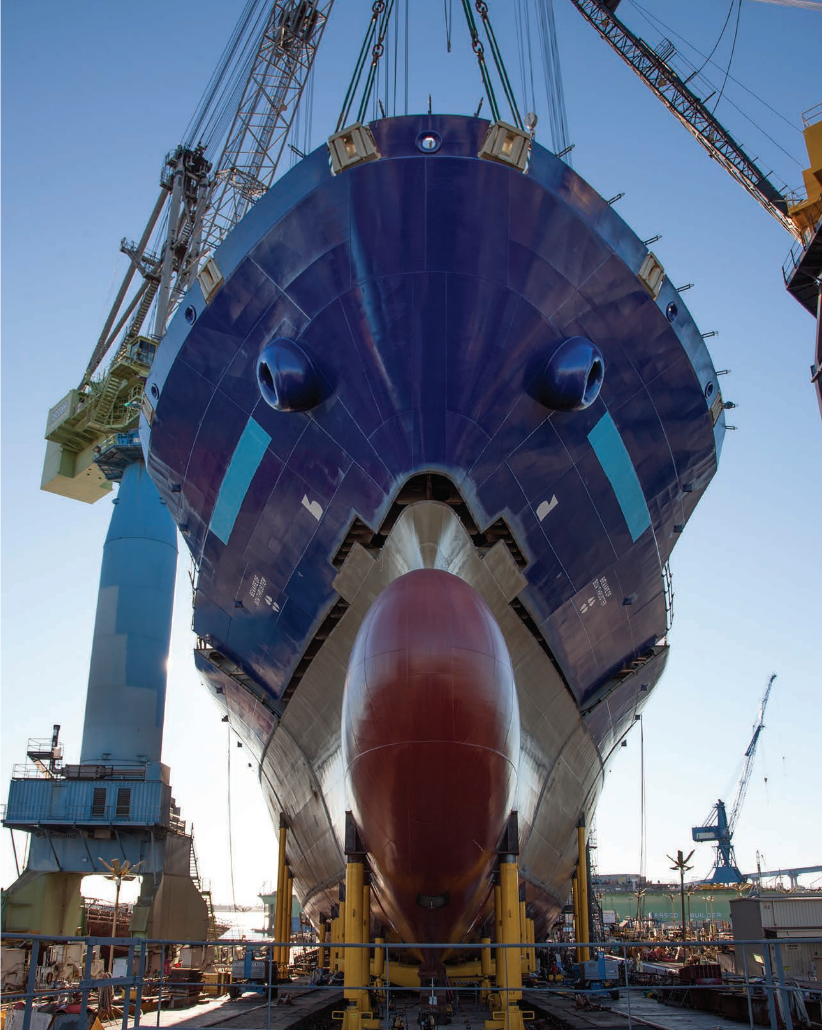
Bow lift for the first LNG-powered containership for TOTE
