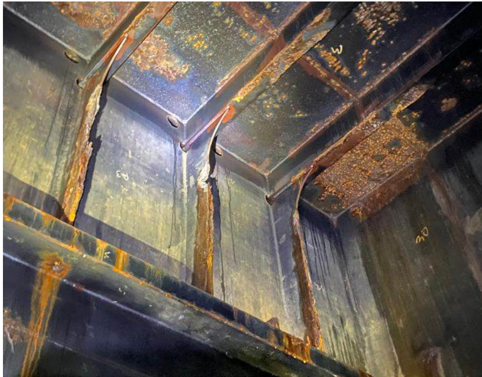
Photo 93 - Tank 6 FWD - P (Fr 31-36): OVHD FBs on OCL WT BHD Sever Notching and Scaling x34
