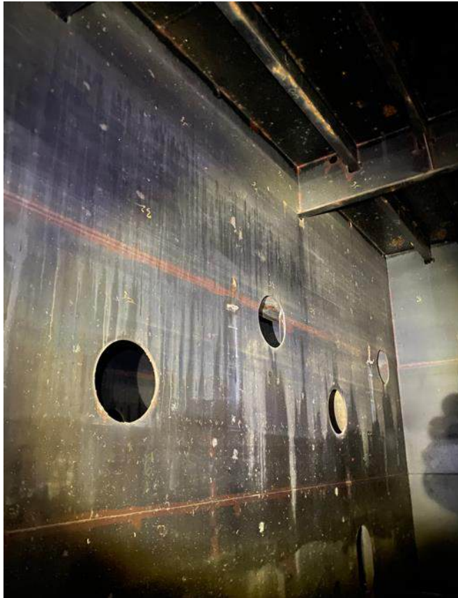
Photo 3 - Typical Condition of Center Ballast Tank
