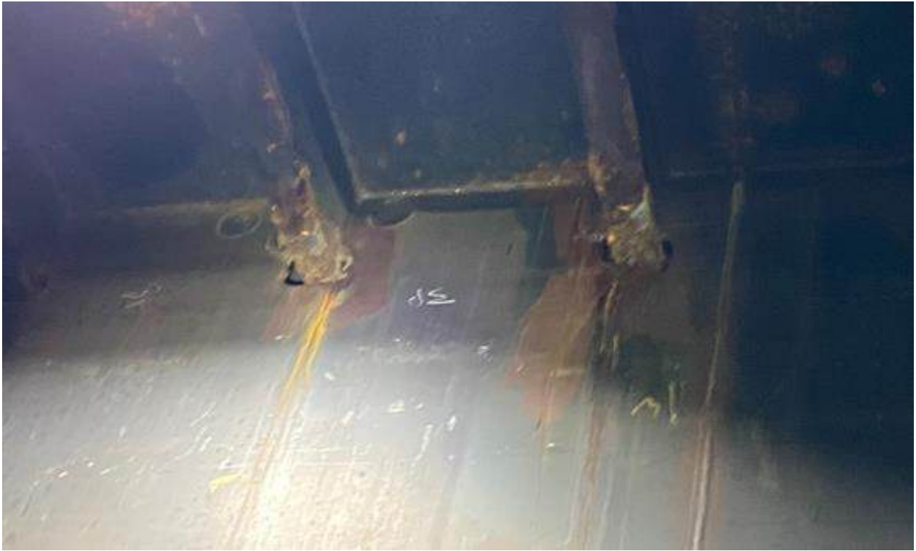
Photo 96 - Tank 6 FWD – PC (Fr 38 & 39): PD Stiffeners Necking IWO OCL WT BHD Pass-thru
