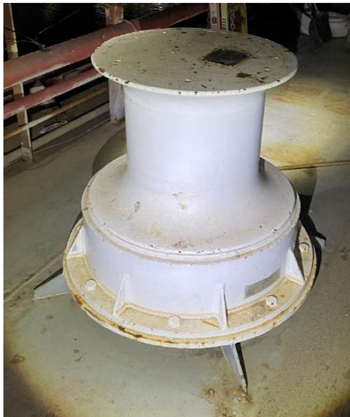
Photo 44 – Typical condition of capstan
