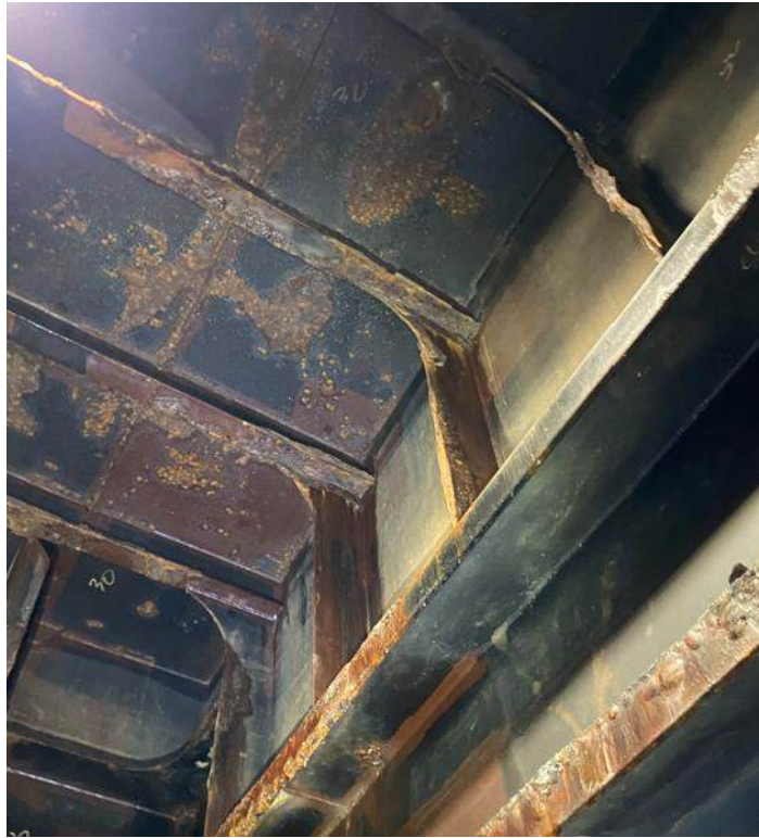
Photo 92 - Tank 6 FWD - P (Frs 37, 38, 40): OVHD FB on OCL WT BHD and PD Stiffenes Scaling/Thinning x33
